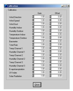
Virtual Weather Station allows you to calibrate for improved accuracy. In addition, if your wind speed sensor is below the expected reading due to bearing life or trees obstructing the anemometer, these errors can be adjusted to provide realistic values.
